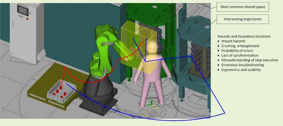
Figure 9 - Cobots in a factory setting
