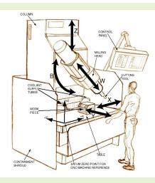
Figure 1 - CNC milling machine
